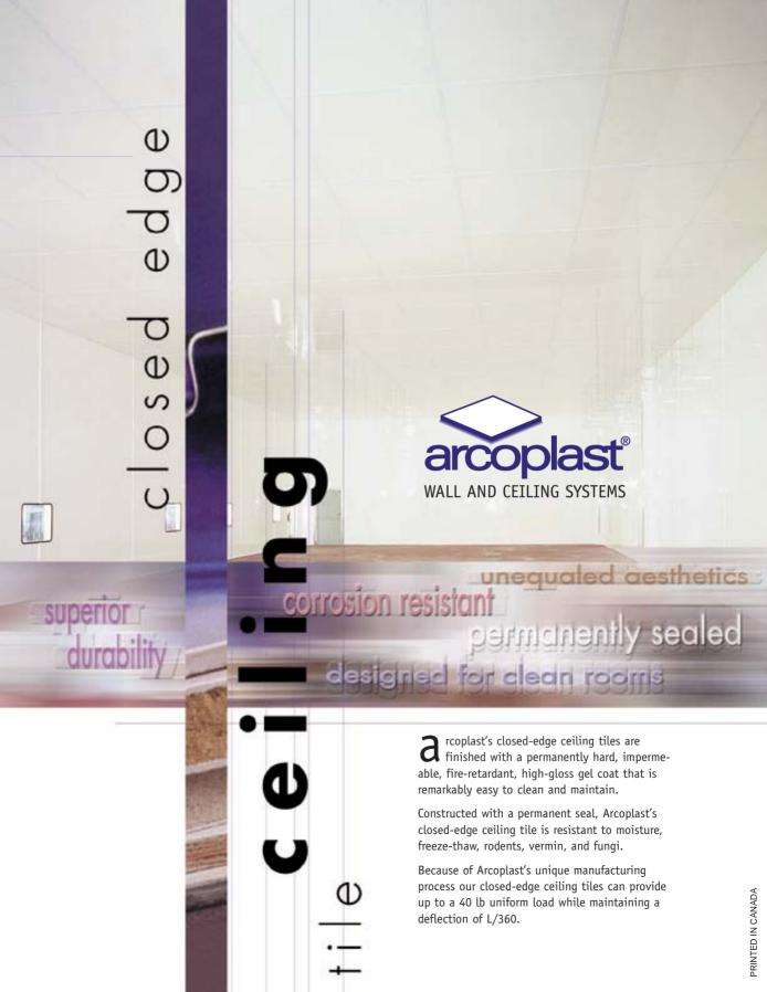
**Tiles:** A foam-core tile layered each side by uniform glass-fiber mat embedded in a fire-retardant resin faced with a gel-coat finish.
